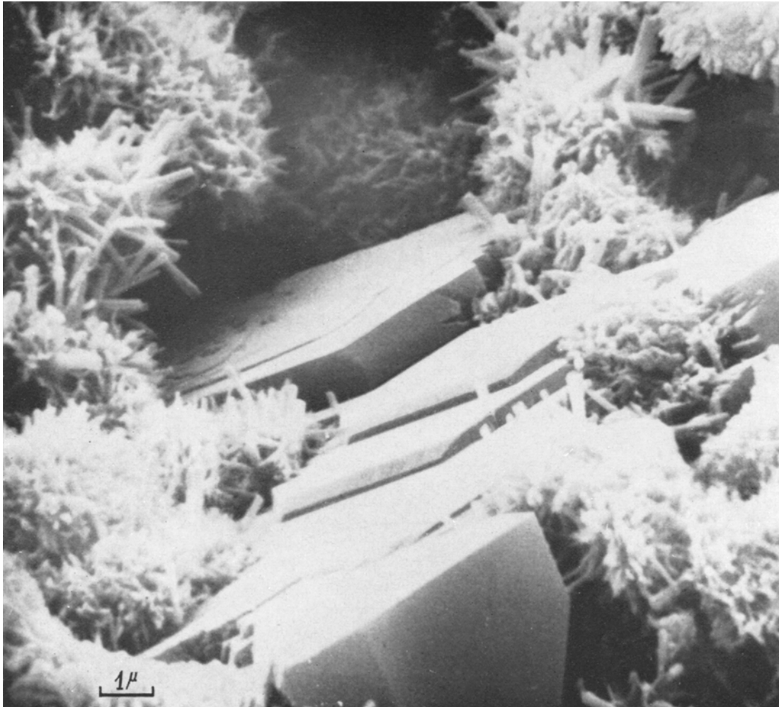
Figure 2 Fracture surface of cement after hydration. (Courtesy of Dr S. Chatterji and Nature [10])
